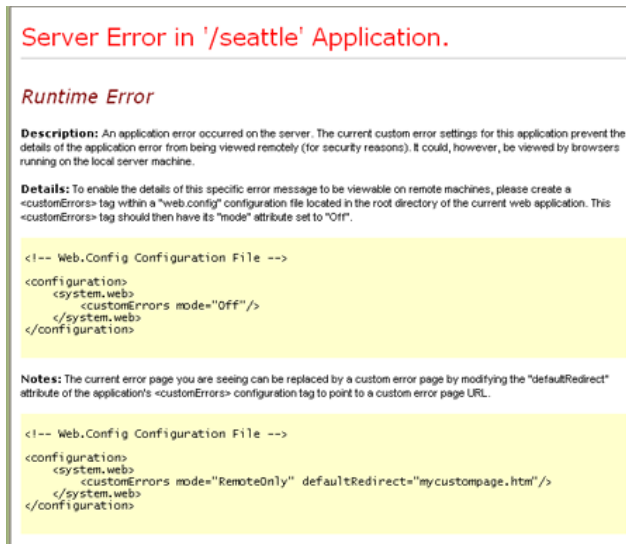
Figure 10: Wrong .NET framework configuration symptom
